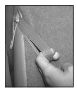
2. Once the latches are engaged, let the seat drop into place. Release the lever labeled 1 and pull the seatback up using the assist strap on the outboard side of the seat to return it to its upright position.
